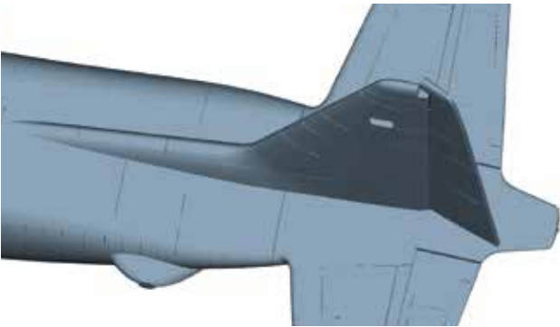
Rudder travel: 10-12mm left / 10-12mm right
